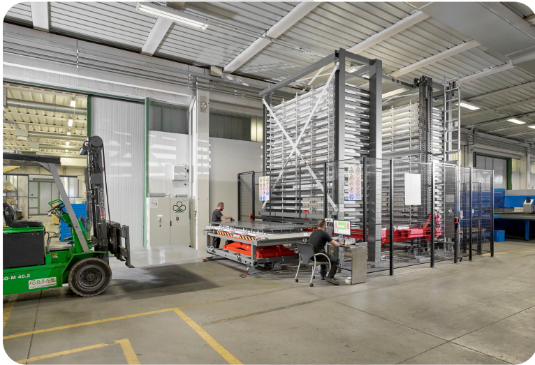
Steel Tower vertical lift module (double tower) For sheet metal
