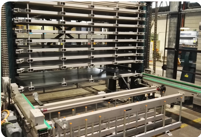
Steel Tower vertical lift module for sheet metal (steel industry)
