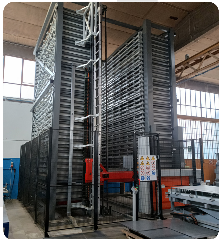
Automated storage system For metal sheets on trays
